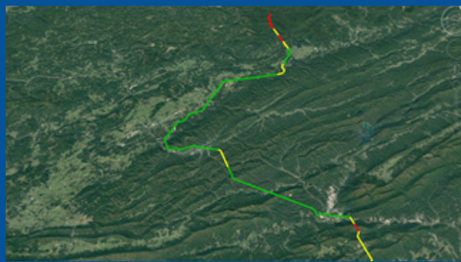
WARP UAS flight plan optimized based on wind speed and direction using micro-scale weather data; shown on Google Earth to highlight terrain-based wind effects
